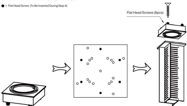
Align pilot holes on the top of the bottom rolling base with the remaining open pilot holes on the large bottom baseplate and screw into place using (6) Flat Head Screws (the screwdriver instead of the drill is recommended for this step).
